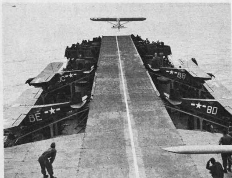
Ramps hold four Cubs as a fifth plane takes off from the narrow runway. On this type, no provision is made for the artillery spotter's return.
